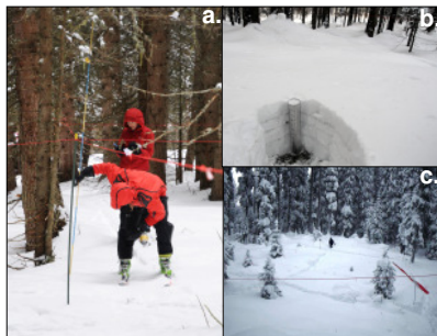
Figure 2. (a) manual snow depth measurements (b) SWE (c) A low canopy closure field area, Laret low with sampling grid.
