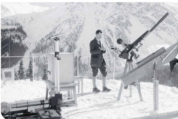
Figure 6: Daniel Chalonge, colleague of F.W. Paul Götz, on the terrace of the 'Firnlicht' house in Arosa in the early 1930s, between the Fabry-Buisson (predecessor of the Dobson spectrophotometer), the Chalonge, and the Féry spectrographs. Photo: unknown. Source: Photo archive MeteoSwiss
